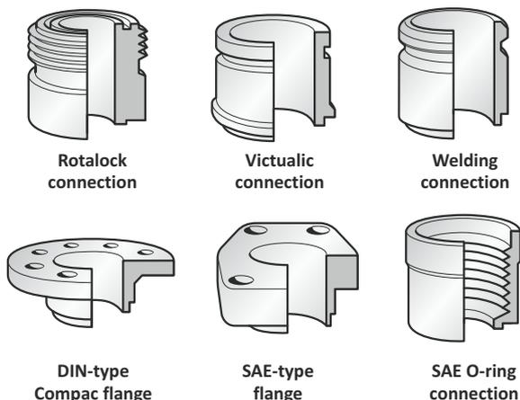
Some connections are equipped with a special plastic cap to protect the connection's threads and sealing surface (X) and to prevent dirt and dust from entering the BPHE. This plastic cap should be removed with care to avoid damaging the thread, sealing surface, or any other part of the connection. Some connections have an external heel whose purpose is to facilitate pressure and leakage testing of the BPHE in production.
