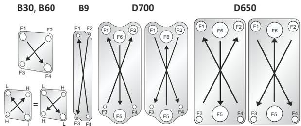
The B9, B30, B60, D650 and D700 have a cross-flow configuration, instead of the parallel flow normally found in BPHEs. In the B9, B30 and B60, ports F1-F4 are equivalent to the outer circuit, and ports F2-F3 to the inner circuit. For the D650 and D700, ports F5-F6 are the outer circuit and ports F1-F4 and F2-F3 are the inner circuits.
