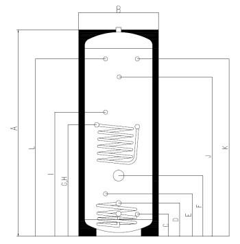
50mm Polyurethane Insulation White Finished Casing Bespoke cylinders available at request
