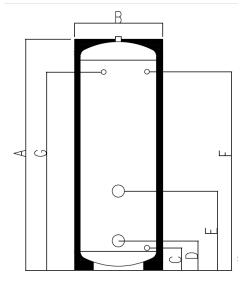
50mm Polyurethane Insulation White Finished Casing Bespoke cylinders available at request
