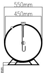
Dimensional Drawing — Horizontal Direct 50mm Polyurethane Insulation White Finished Casing
