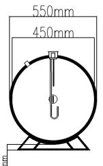
Dimensional Drawing — Horizontal Direct 50mm Polyurethane Insulation White Finished Casing
